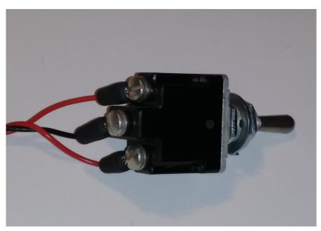
**NOTE:** (Emergency Lights Toggle) Connect pin 25 (OFF position) to toggle terminal #1 and common line (ARM position) to toggle terminal #2. If emergency conditions are met, Relay 16 will close and the Emergency lights will activate. Use second pole for manual selection to the ON position. Connect 12 volt power to toggle terminal #6 and ground to toggle terminal #5 from LEFT HOT BUS to the Emergency Lights in cabin.
