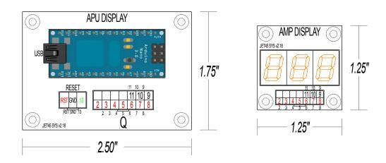
**NOTE:** PLUG "Q" is connected to an isolated Arduino Nano to operate the APU AMP Window comprised of three Vishay seven segments displays via Multiplexing
