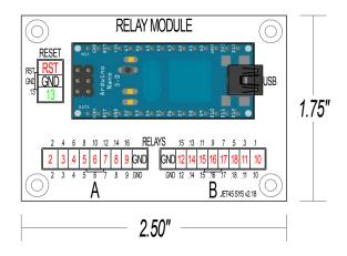
**NOTE:** The 16 Relay Module enables software simulation to physically control hardware components within the cockpit, in some cases, hardware requiring 5v or 12v power.
