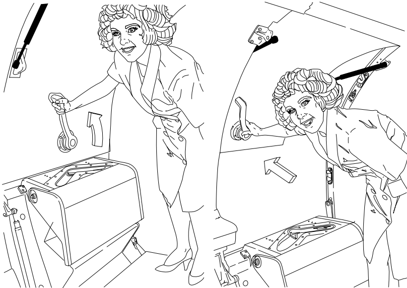
LEFT FORWARD EMERGENCY EXIT OPERATION
