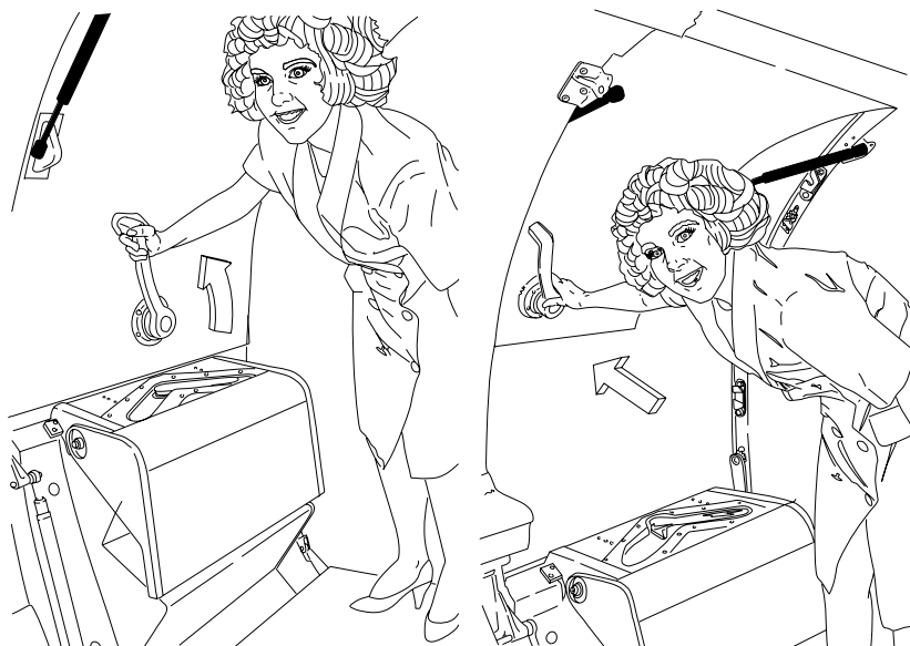
LEFT FORWARD EMERGENCY EXIT OPERATION
