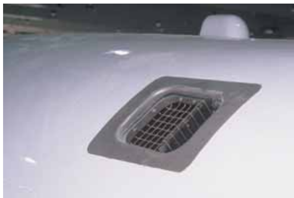
Figure 16a—APU Inlet (if installed) Clear of obstructions
