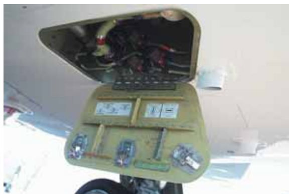
Figure 7g—Fuel Drains and Access Door Drain if contamination is suspected and secure
