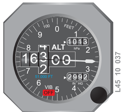
Figure 42 - Standby Barometric Altimeter
