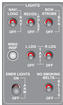
Figure 3m—All Exterior Light Switches (if night flight is anticipated) On. Check proper illumination All Exterior Light Switches OFF
