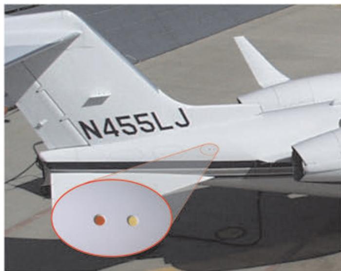
Figure 4 - Fire Bottle Discharge Indicators
