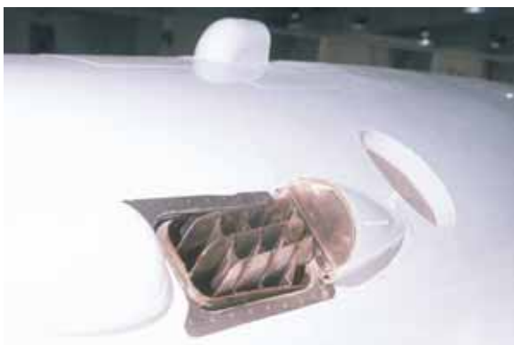
Figure 14d—APU Exhaust (if installed) Clear of obstructions
