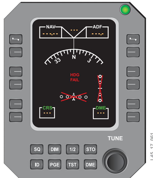
Figure 9 - Standby Navigation Display Failure Indications
