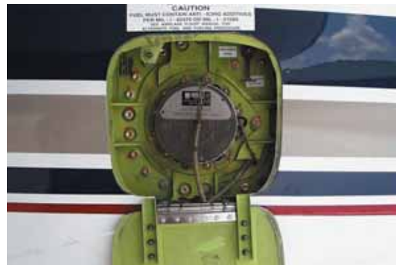
Figure 12b—Single-Point Fueling Access Doors Secure
