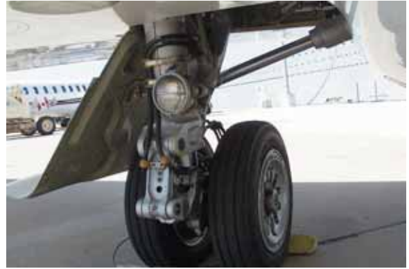
Figure 7i—Right Main Gear Check: wheel well, hydraulic/fuel leakage—condition; taxi light and lens—condition; wheels, brakes, and tires—condition; main gear strut—check proper extension
