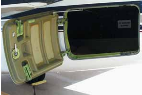
Figure 16d—Baggage Compartment Door Open: baggage heat switch—on, as desired; check condition of door seal, then close
