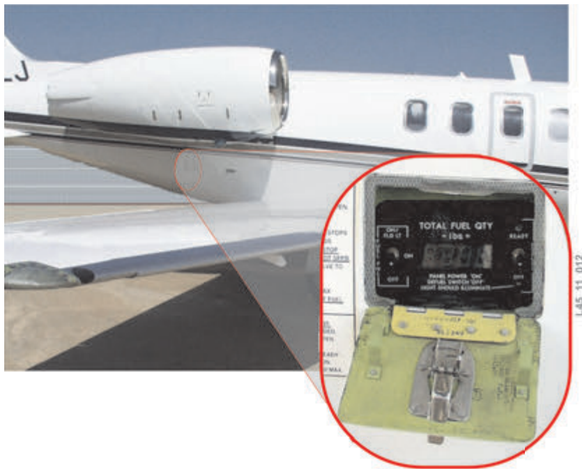
Figure 8 - Refueling Control Panel
