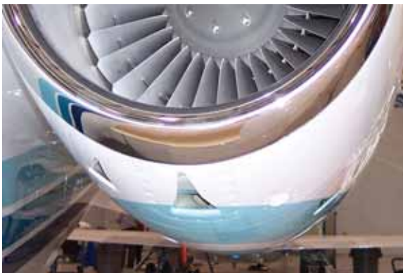
Figure 22d—Left Generator and Alternator Cooling Scoops and NAC bleed outlet Clear
