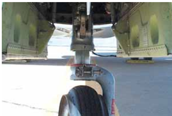
Figure 4d—Ground Wire Disconnected
