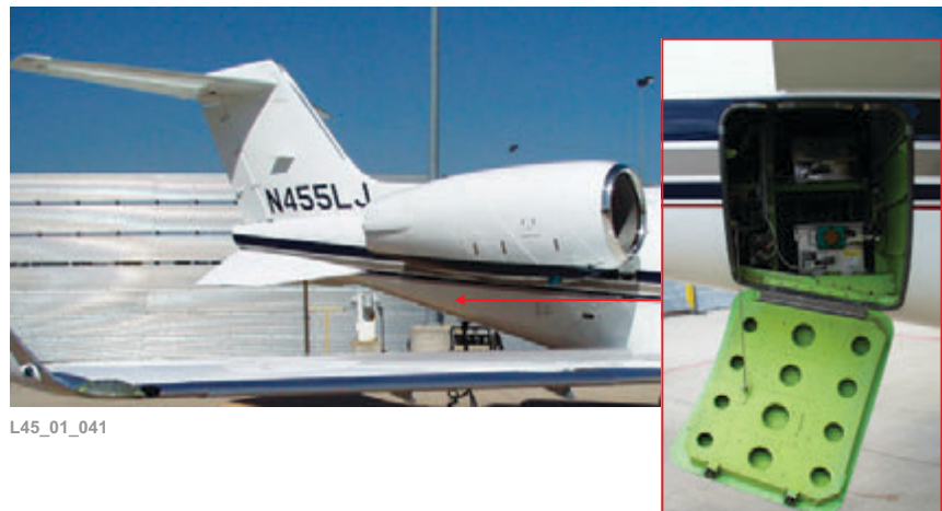
Figure 11 - Equipment Bay Door
