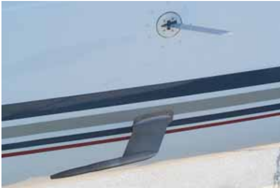
Figure 1a—Left Pitot-Static Probe Cover removed, clear of obstructions Stall Warning Vane Freedom of movement Ice Detect Probe
