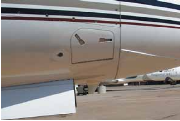
Figure 6b—Oxygen System Discharge Indicator and Service Door Check and secure
