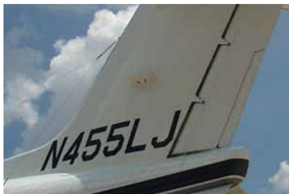
Figure 16b—Left VOR/LOC Antenna Condition
