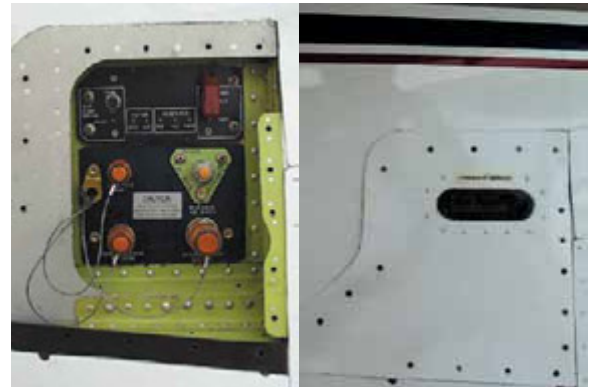
Figure 12a—Hydraulic Service Panel Check FILTER (MAIN or AUX) and reservoir (ADD or OVER) lights not illuminated. Access panel secure.
