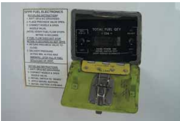
Figure 12c—Fuel Quantity Panel Access Door Secure
