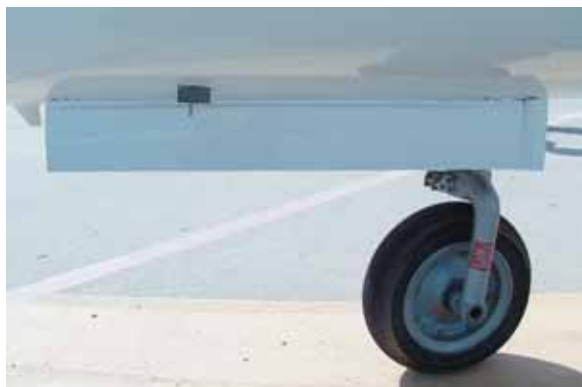
Figure 4c—Nose Compartment Doors, Wheel, and Tire Condition and nose gear uplock forward
