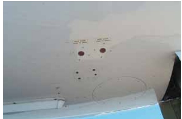
Figure 6e—Standby Pitot and Static Drains Push up to drain. Required if moisture is known or suspected.
