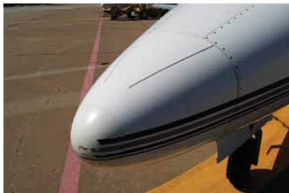
Figure 5a—Radome and Radome Erosion Shoe Condition
