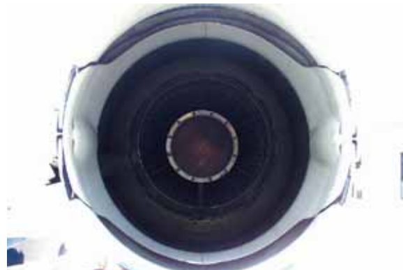
Figure 13a—Right Engine Turbine Exhaust Area Condition, clear of obstructions
