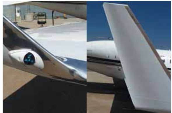
Figure 9a—Right Winglet NAV Light/Lens and Static Wicks (4) Condition
