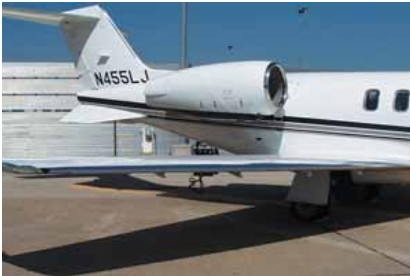
Figure 8a—Right Wing Check: Leading edge, stall strips, triangles, vortilons, and ice detect patch—condition; access panels—fuel/hydraulic leakage
