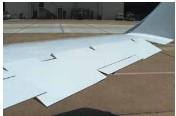
Figure 10a—Right Aileron Check free motion, balance tab linkage, and brush seal condition
