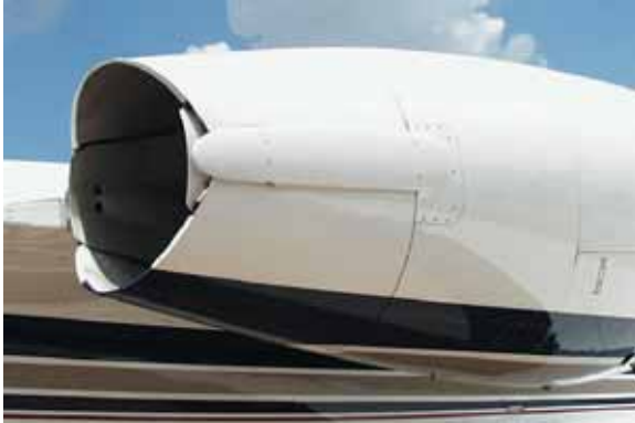
Figure 13b—Right Thrust Reverser Condition and completely stowed
