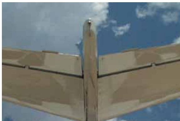
Figure 15c—Beacon/Strobe Light and Lens Condition
