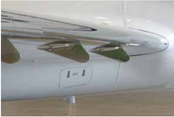
Figure 7h—Toilet Servicing Door Secure
