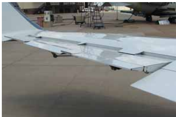
Figure 19b—Left Aileron Check: free motion, balance, and trim tab linkage and brush seal condition
