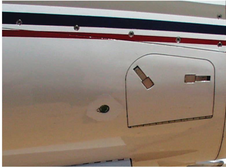
Figure 6 - Oxygen Overboard Discharge Indicator
