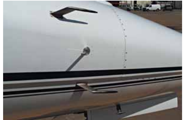
Figure 2a—Right and Standby Pitot-Static Probes Cover removed, clear of obstructions Stall Warning Vane Freedom of movement
