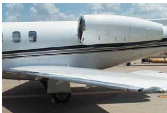
Figure 21a—Left Wing Check: leading edge, stall strips, triangles, vortilons, and ice detect patch—condition; access panels—fuel/hydraulic leakage
