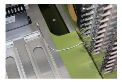
These metal parts are **bonded** together, but they are not necessarily grounded.
