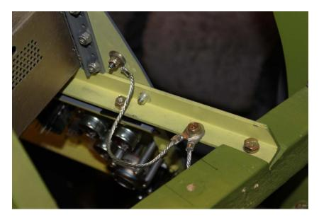
Here, the left side of the main instrument panel is **bonded** to the switch panel structure.
