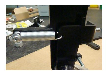
At this point you could insert the small return spring into the toe pedal bracket as shown here before you attach the pedal to the rudder arm,look at the pic below of the spring one end will be cut open and goes to the toe pedal bracket, cut it like in the picture the closed end will go to the rudder arm machine screw.
