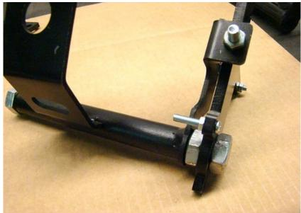
Notice the 1" X 8/32 machine screw at the bottom edge of the rudder arm, insert it as shown here, this is the toe pedal stop bolt.
