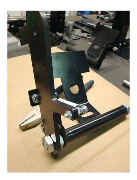
Now flipped around the other way, find the 5/8" X 7" bolt and 2 5/8" jam nuts. The idea here, is to get the pedal tube as tight as you can between the bolt head and the first jam nut, yet still allow the pedal to swing freely with no resistance. The best way to do that is to run the jam nut up against the tube end then back it off a hair, install the other jam nut on the other side, and tighten both nuts together it might take you a couple of tries to get it just right.
