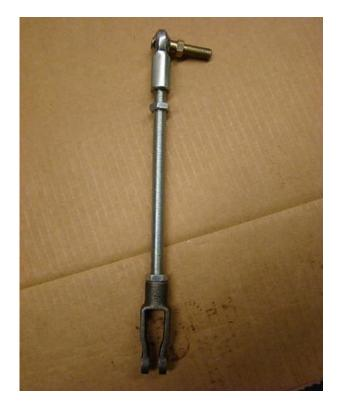
Next linkage pushrod connection, your linkage rod should look like this 1 jam nut for the spherical rod end and 1 for the clevise end after adjustment you tighten down the jam nuts.
