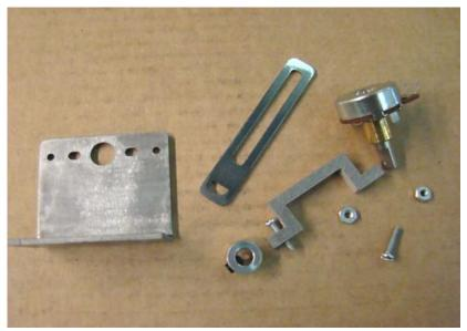
Find these pieces, the pot is the same pot used in the CH Rudder pedals you can get from the CH website the HP-100A
