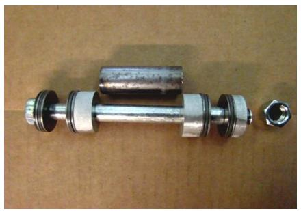
Ok find the 7/16" X 4 5/8" long bolt, arrange like this starting from the bolt head, 1 black washer,1 bearing set, the rudder arm next,1 bearing set, 3/8 aluminum spacer, at the top hole in the square post, insert the 1 3/4" steel spacer, then run the bolt and rudder arm through the square tube and steel spacer, next on the other side will be a 3/8" aluminum spacer, a bearing set, the other rudder arm, a bearing set, and a 1/4" aluminum spacer and the nylock nut.
