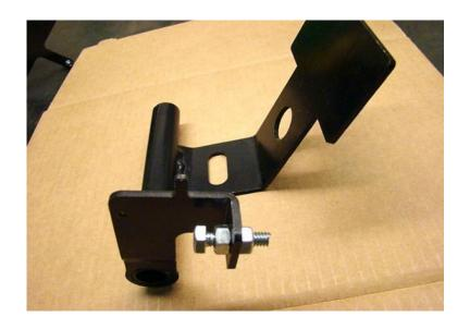
There is a left and a right rudder pedal,im sure you will figure out which one is which, grab a left and right pedal, find 2 7/16" X 1" bolts and 4 nuts, insert the bolts as seen here into the toe pedal adjuster bracket, these bolts are used to adjust the toe pedals in or out to your liking.
