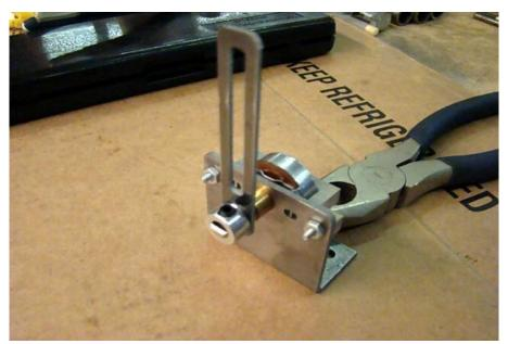
Assemble as per picture, the connections will be straight down on the backside, push the collar on tight against the swing arm and tighten the set screw.
