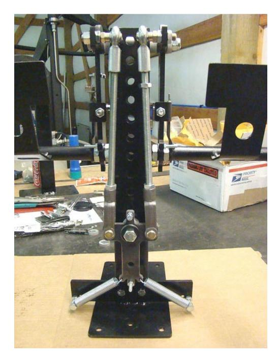
Here is basically what you should have now. You can attach the bigger springs now,again cut one end open for the bellcrank side the other end leave closed.
