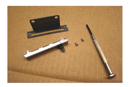
Next you can attach the slide pot to the bracket, make sure when you order your pot that you order the screws also, they don't come with the pot. Also you may want to put a small washer on the screw to bring the screw out a little bit I noticed that it went into far and wouldnt allow the slide arm on the pot to fully retract all the way closed, so you might check that when you put it together.
