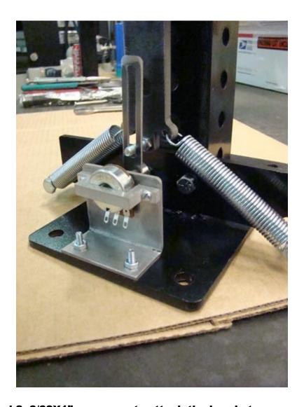
Find 2 8/32X1" screws nuts,attach the bracket as you see it here, the panhead of the screws will be on the bottom, dont worry those will sit down in the holes that are cut in the top aluminum shim plate that goes underneath,the main base,you see here.
